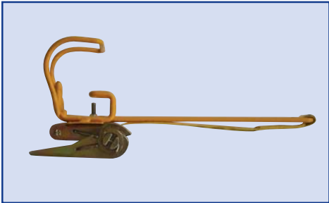
Expanding ratchet to tighten panel against the wall to ensure stability
